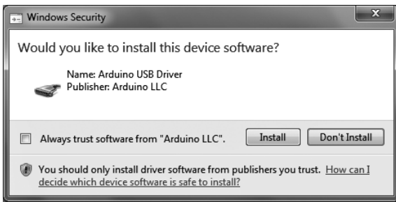
Figure 19.8 Option to select a USB driver for use with the IDE package
