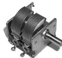
Figure 2.34 An air-spaced variable capacitor. This component (used for tuning an AM radio) has two separate variable capacitors (each of 500\ \text{pF} maximum) operated from a common control shaft
