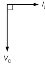
Figure 4.7 Phasor diagram for a pure capacitor
