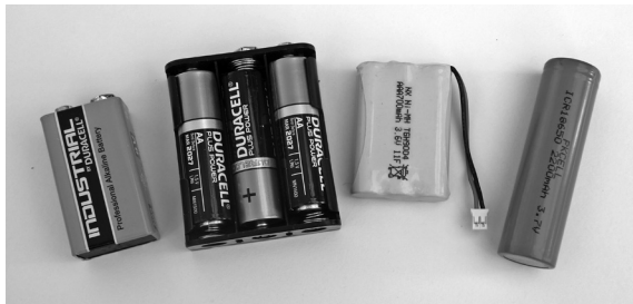
Figure 6.32 Some typical battery packs for small electronic equipment. From left to right: alkaline a 9 V PP3 based on six layered 1.5 V cells; a 4.5 V battery pack based on three 1.5 V alkaline cells; a 3.6 V pack based on three Ni-MH cells; a single 3.7 V high-capacity Li-ion cell.
