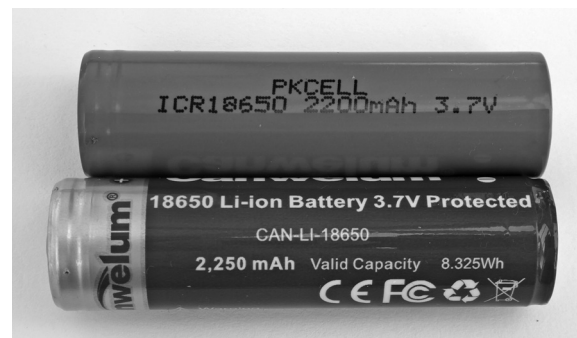
Figure 6.35 Protected (bottom) and unprotected (top) 3.7V 18650 cells
