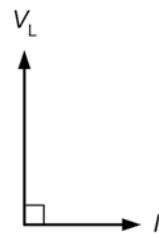
Figure 4.10 Phasor diagram for a pure inductor
