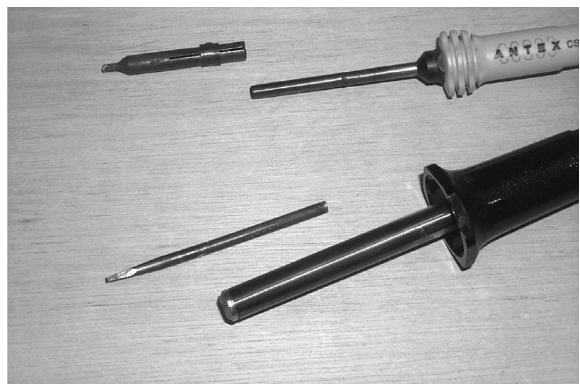
Figure 20.18 Two different types of bit fitted to small soldering irons
